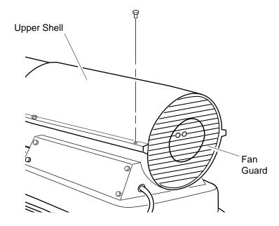
Figure 5 - Upper Shell Removal, 100,000 BTU/Hr Model
